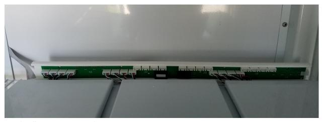
Load Cell Connector Board
