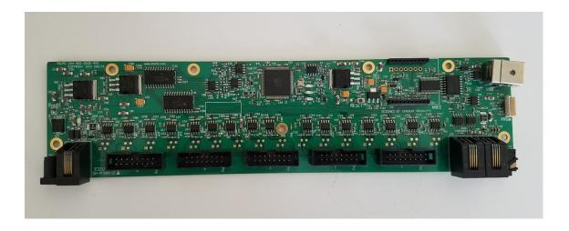
If you have 5 rows of shelves, a fifth flat cable can be placed into connector three and the corresponding port layout will be [16, 15, 14], [12, 11, 10], [13, 9, 5], [8, 7, 6], [4, 3, 2].
